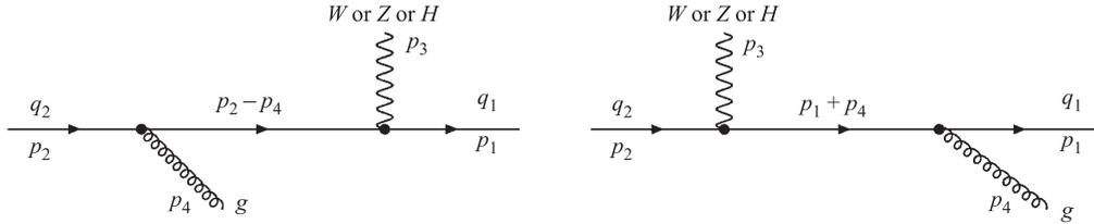
Fig. 3. Gluon bremsstrahlung from two quark legs
