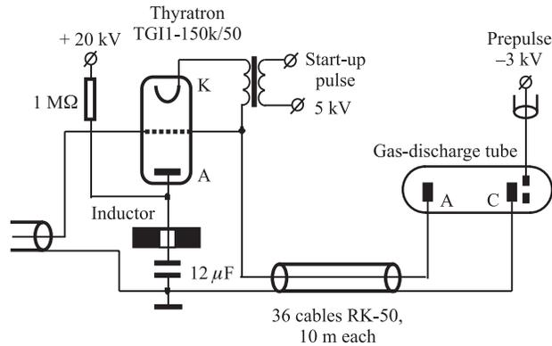
Fig. 2. Functional scheme of the current generator for the plasma lens
