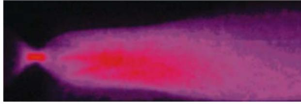
Fig. 6. Temporal scan of the plasma emission for the initial argon pressure of 3.5 mbar and the discharge current of 200 kA; the total scan duration is 6  $\mu$ s, the transverse size is 2 cm
