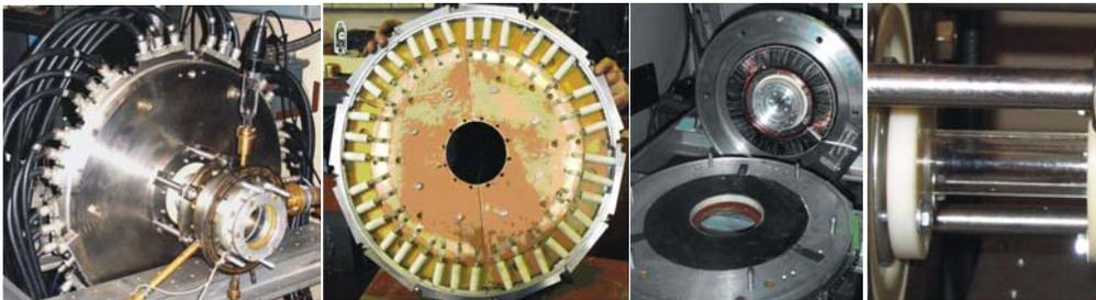
Fig. 4. Plasma lens units: general view of the plasma lens on its test bed (on the left), the current receiving section, the inner part (Rogovskii coil around the anode cup), the cathode unit with the gas-discharge tube (on the right)
