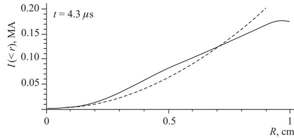
Fig. 8. Total current inside a radius as a function of this radius. Dashed curve corresponds to a uniform current-density distribution
