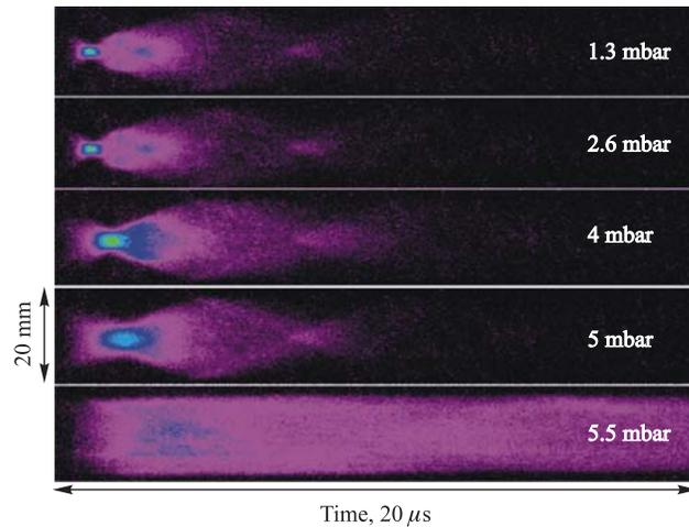
Fig. 5. Plasma pinch dynamics at different argon pressures,  $J = 80 \text{ kA}$
