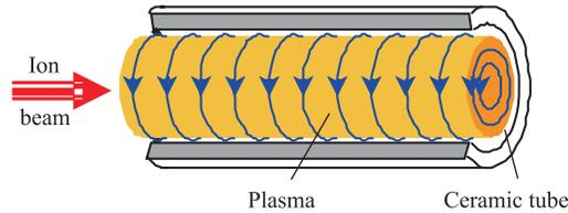
Fig. 1. Ion focusing in a plasma lens
