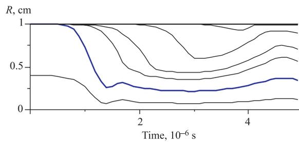
Fig. 7. Trajectories of radial plasma motion. The interface between the argon and the wall-material plasma parts is shown as a thick line
