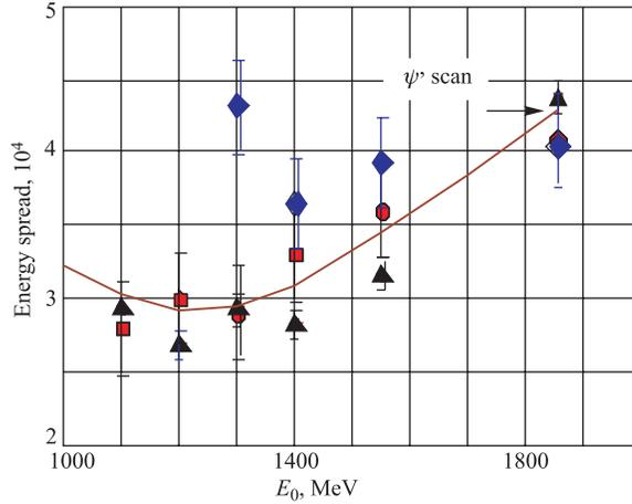
Fig. 6. Variation of the beam energy spread depending on the beam energy.  $\blacklozenge$  — CBS data;  $\blacktriangle$  — method (III) data;  $\bullet$  — method (II) data; curve — simulation results. The arrow shows the data of the KEDR detector
