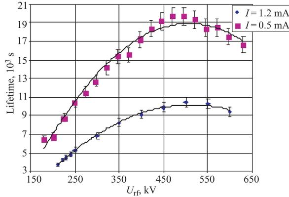
Fig. 5. The dependence of the beam lifetime on accelerating voltage
