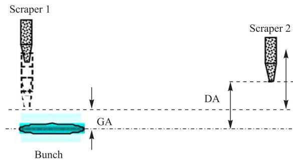
Fig. 1. GA — geometrical aperture dependent on the transverse coordinate of scraper 1; DA — dynamical aperture, measured with dependence of the beam lifetime on transverse coordinate of scraper 2. The case of  $GA < DA$  is shown
