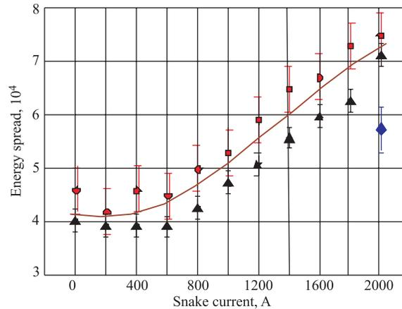
Fig. 7. The beam energy spread depending on the snake current.  $E_0 = 1855$  MeV, the same symbols as in Fig. 6
