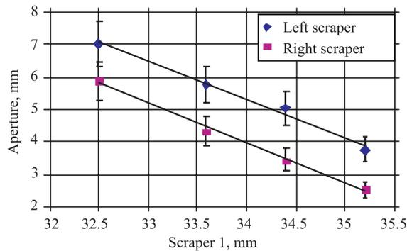
Fig. 2. Dependence of the aperture measured by scraper 2 at the insertion depth of scraper 1
