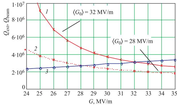
Fig. 2. External coupling (1, 2) and beam load (3) vs cavity gradient
