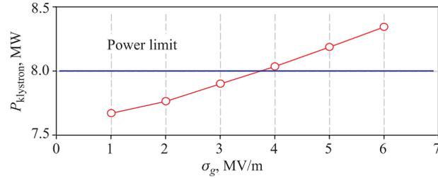
Fig. 7. Total klystron RF power vs gradient spread (average gradient is 31.5 MV/m)
