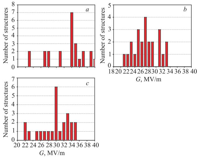
Fig. 4. Accelerating cavities maximum gradients distribution (based on experimental data). a) 3rd production EP ( $Q_0 = 10^{10}$ ); b) 4th production EP ( $Q_0 = 10^{10}$ ); c) modules ACC (5, 6, 7). Beam: ON
