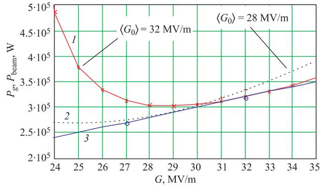
Fig. 3. Input power (1, 2) and beam power (3) vs cavity gradient
