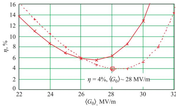
Fig. 6. Total power loss vs matched gradient (solid line — experimental gradients spread, dashed line — asymmetrical Gaussian distribution)
