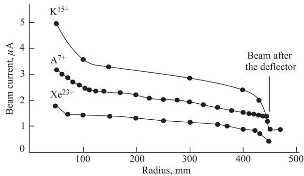
Fig. 4. Beam current distribution during acceleration of Ar, Kr, and Xe ions
