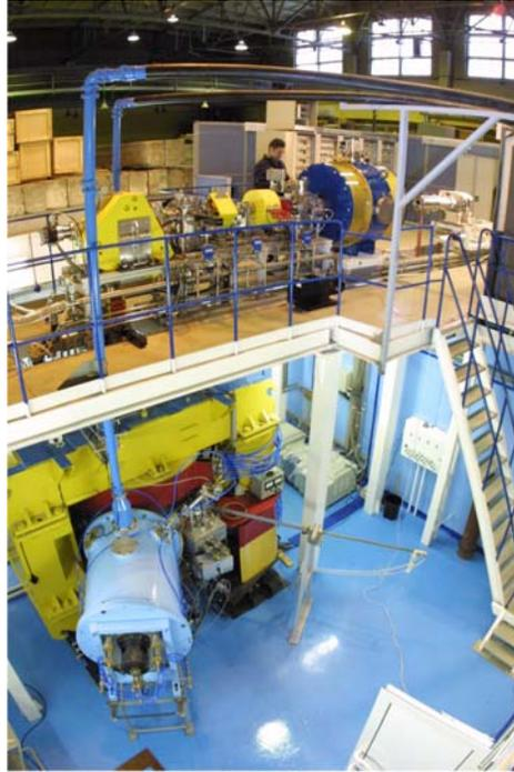
Fig. 1. IC100 cyclotron. Shown are the SC ECR source, injection line, magnet and resonance cavity
