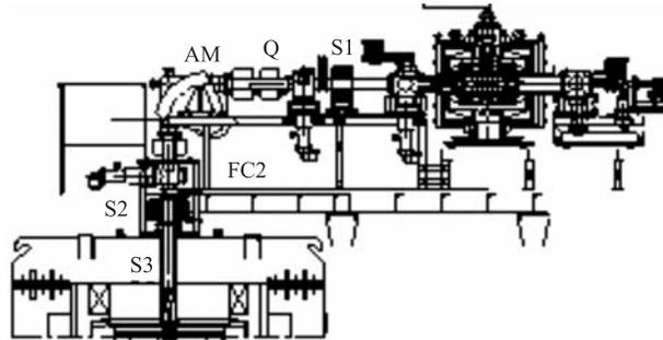
Fig. 3. Axial injection channel (length  $\approx 5 \text{ m}$ ). DECRIS — superconducting ECR ion source; AM — analyzing magnet; S1, S2, S3 — focusing solenoids; Q — correction quads; FC2 — Faraday cup
