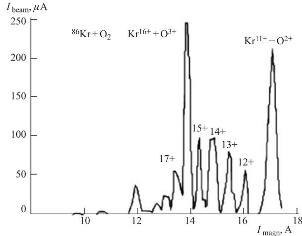
Fig. 2. Kr spectrum from DECRIS-SC. Extraction voltage is 12.5 kV. SRF power is 380 W
