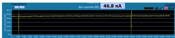
Fig. 7. Long-term stability of  $^{132}\text{Xe}^{23+}$  beam. Current was measured on target. Irradiation period 1 h
