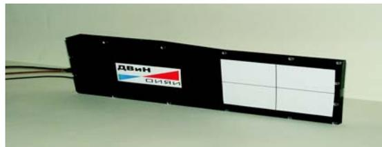
Fig. 5. The profilometer to measure spatial distributions of the neutron tagged beams. The working area is marked by the white sheet with the cross
