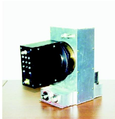
Fig. 3. The box of the frontend electronics of the alpha detector mounted on a neutron generator with ground target
