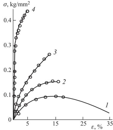
Fig. 11. Uniaxial tensile stress-strain curves  $\sigma$  at the deformation rate  $d\varepsilon/dt = 3.3 \cdot 10^{-4} \text{ s}^{-1}$  on a polycrystal  $\text{CH}_4$ : 1)  $T = 77$  K; 2)  $T = 64$  K; 3)  $T = 20$  K; 4)  $T = 4.2$  K
