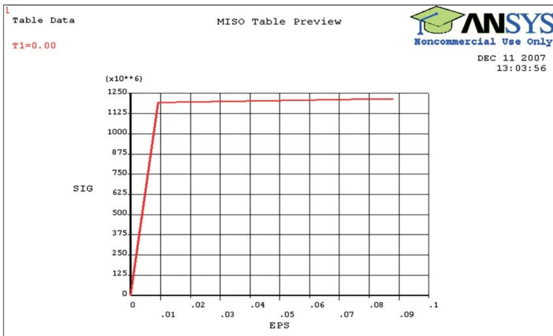
Fig. 5. Stress-strain curve for Grade-2 Titanium at 4 K
