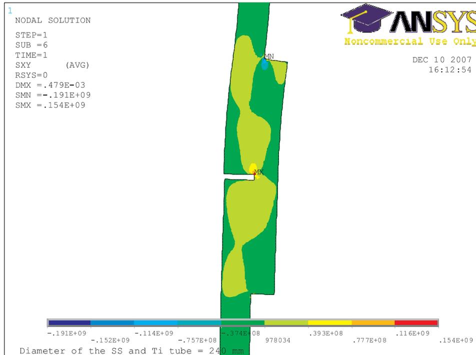
Fig. 11. Shear stress  $XY$  for the case II
