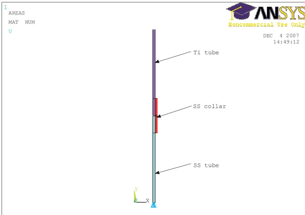
Fig. 4. FEA model of the bimetallic transition joint
