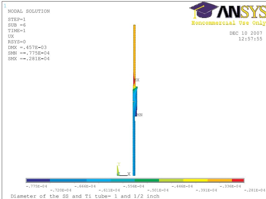
Fig.6. Deformations along the  $X$  direction for the case I
