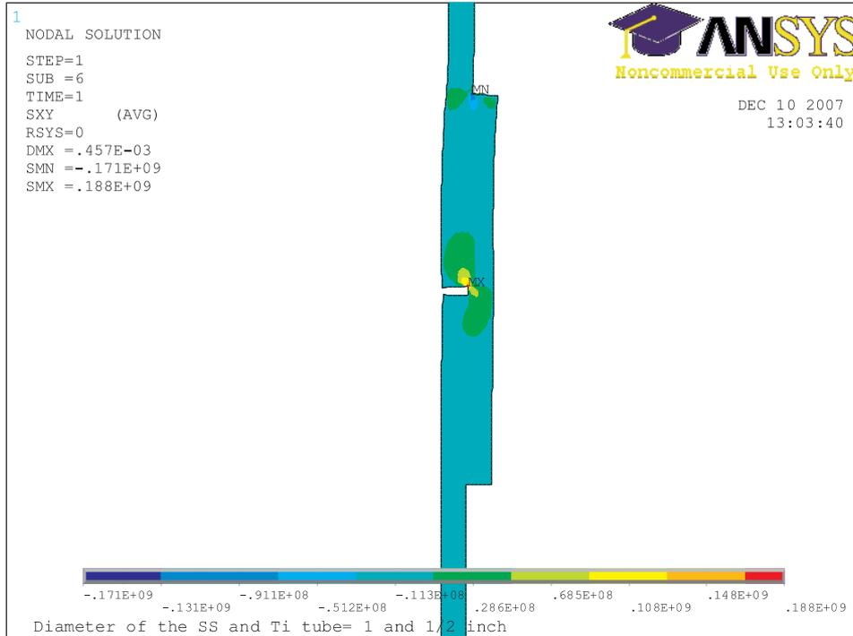
Fig. 10. Shear stress  $XY$  for the case I
