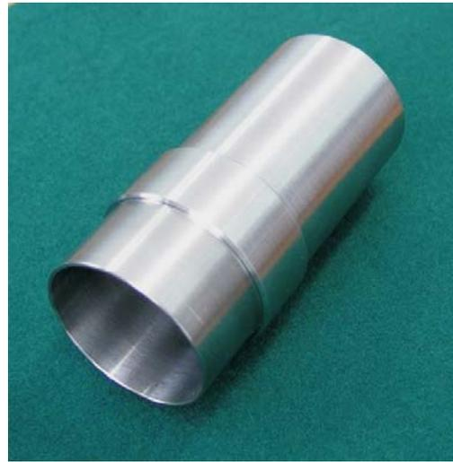
Fig. 1. The bimetallic (Ti–SS) transition joint produced in Sarov with 1.5 inch diameter pipes
