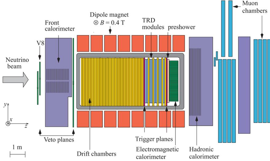
Fig. 5. A side-view of the NOMAD detector
