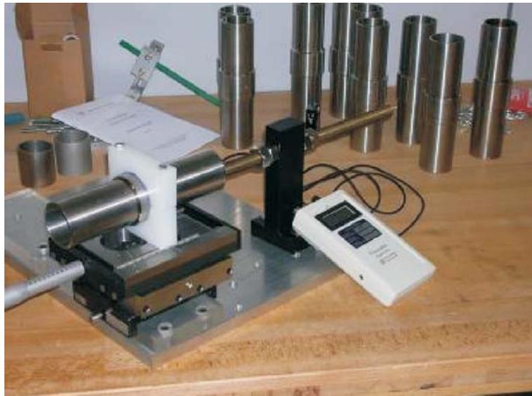
Fig. 7. Tools to measure the residual magnetic field inside the tubes
