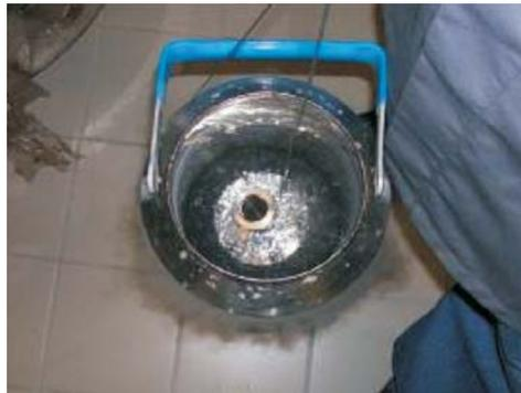
Fig. 5. A sample dipped in liquid nitrogen within a Dewar
