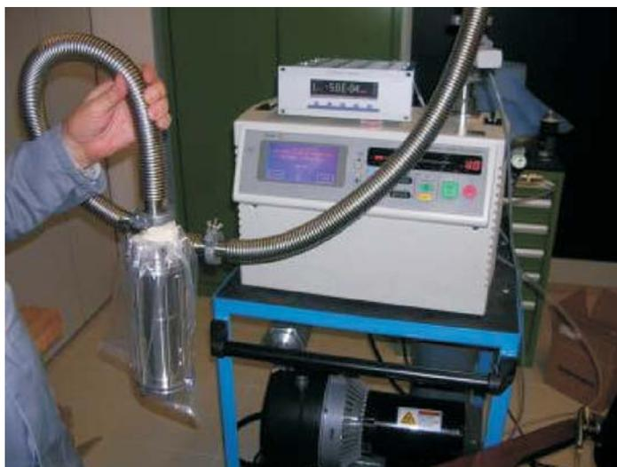
Fig. 4. The Ti-SS transition joint wrapped with a plastic bag for the He leak test measurements
