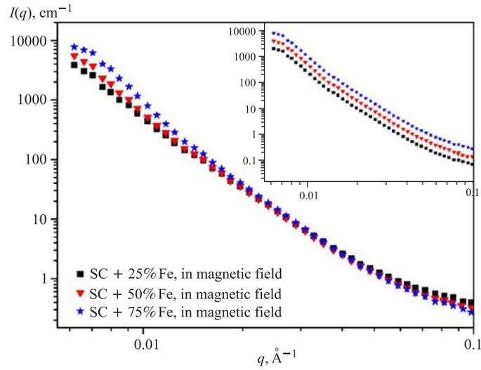
Fig. 6. Experimental curves for magnetic elastomers polymerized in magnetic field,  $B = 156.5$  mT. Inset graphs show the same curves scaled down by a factor of 2 for 50% Fe and by a factor of 4 for 25% Fe, as compared to curve for 75% Fe concentration
