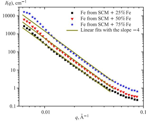
Fig. 8. Scattering curves for magnetic elastomers with various Fe concentrations ( $B = 156.6$  mT, only Fe particles contribution)
