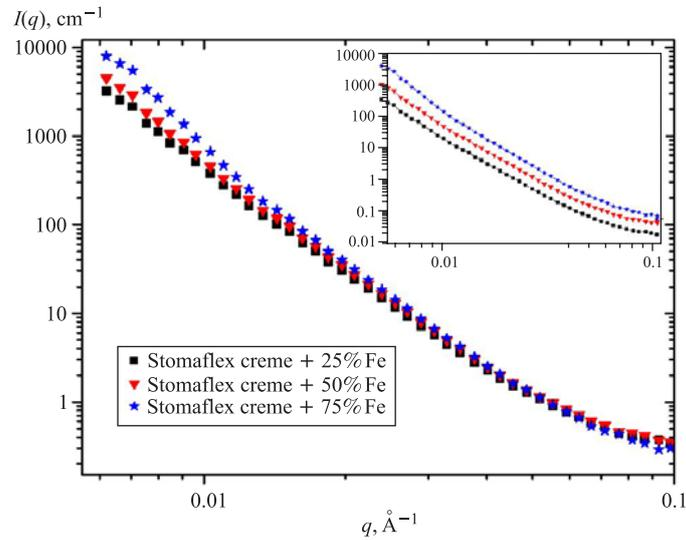
Fig. 5. Experimental curves for magnetic elastomers polymerized in zero magnetic field. Inset graphs show the same curves scaled down by a factor of 2 for 50% Fe and by a factor of 4 for 25% Fe, as compared to curve for 75% Fe concentration
