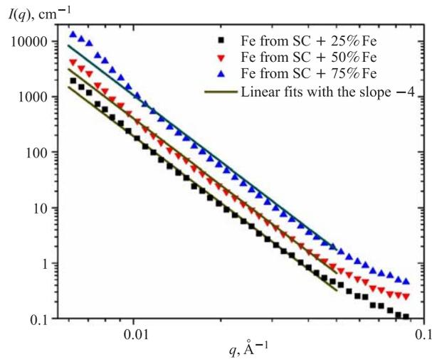
Fig. 7. Scattering curves for magnetic elastomers with various Fe concentrations ( $B = 0$ , only Fe particles contribution)
