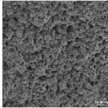
Fig. 2. Stomaflex creme + 75% Fe particles
