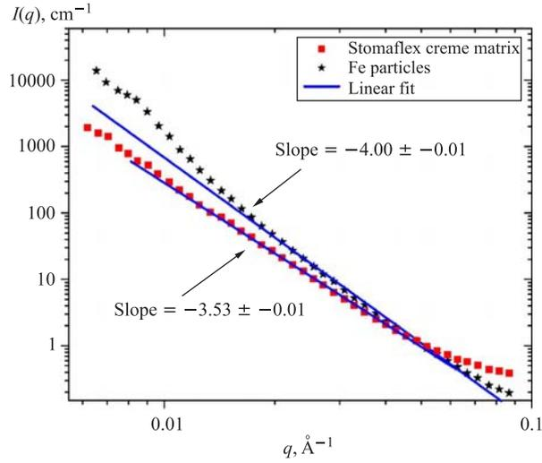
Fig. 4. Experimental curves for Fe particles, polymer matrix and linear fits
