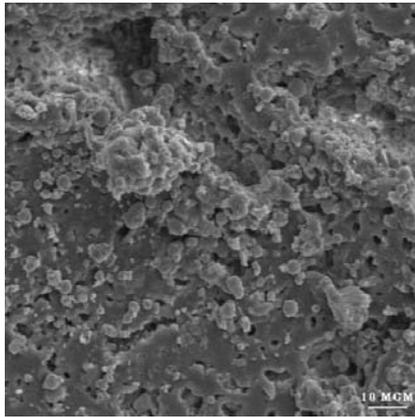
Fig. 1. Stomaflex creme + 25% Fe particles
