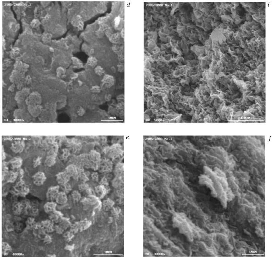
Fig. 3. SEM images of two samples containing iron oxide nanoparticles obtained by means of two different methods; sample A (*a–e*) and sample B (*f–j*)
