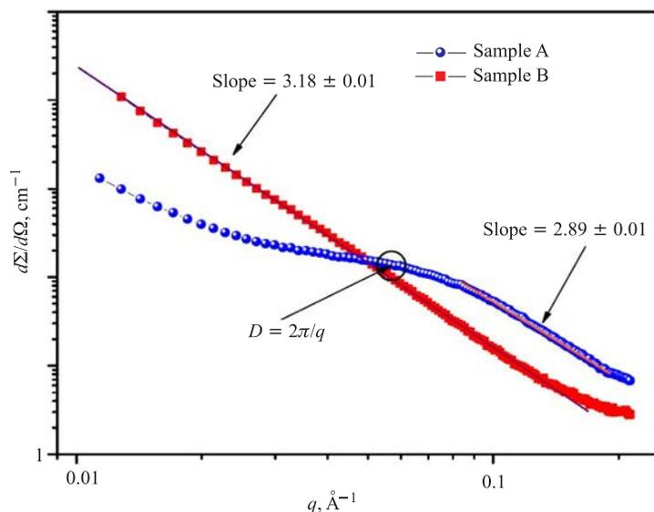
Fig. 5. SAXS experimental curves from samples A and B obtained at Bruker Nanostar SAXS spectrometer in function at the Institute of Synthetic Polymer Materials RAS, Moscow
