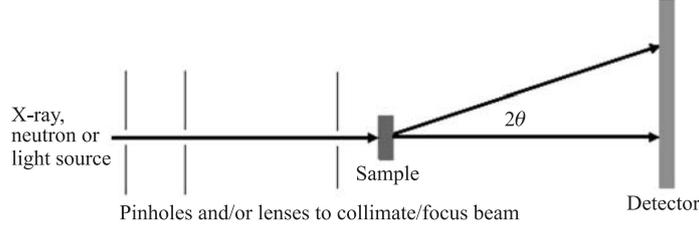
Fig. 4. Representation scheme of the small-angle scattering setup
