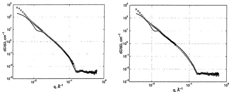
Fig. 14. Results obtained by the fitting of the measured small-angle neutron scattering spectra of the polydispersed population of the ceramide 6 / cholesterol / palmitic acid / cholesterol sulfate unilamellar vesicles at a temperature 32°C (left panel) and 60°C (right panel) in the framework of the separate-form-factor method within the hydrophobic-hydrophilic approximation. The fitting was performed in the range of scattering vectors  $q \geq 0.02 \text{ \AA}^{-1}$
