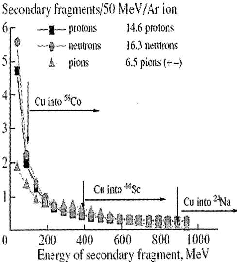
Fig. 12. Calculated energy spectra for secondary protons, neutrons and pions produced by 72 GeV  $^{40}\text{Ar}$  in thin Cu target using the Dubna DCM code
