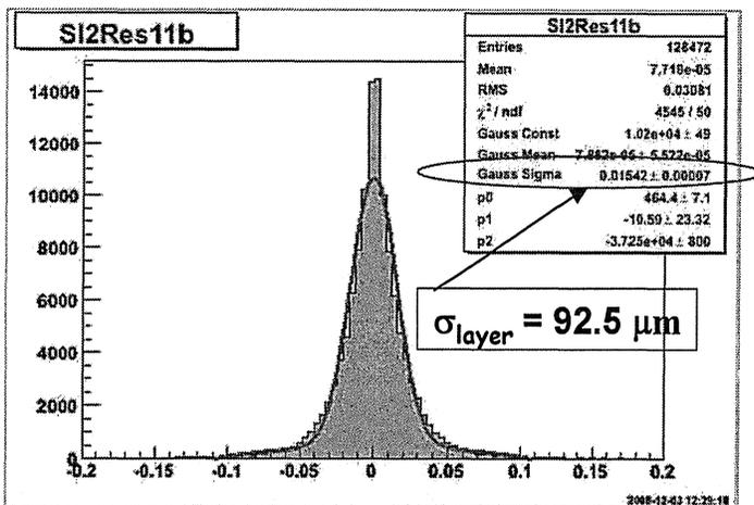
Fig. 9. Dubna Cathode Strip Chamber (CSC) Single Layer Spatial Resolution from Muon Cosmic Data (CMS, LHC). CMS Technical Proposal requirement for Dubna CSC spatial resolution:  $\sigma(\text{CSC}) = 75 \mu\text{m}$ , obtained  $\sigma(\text{CSC}) = \sigma_{\text{layer}} / (\text{number of Degrees of Freedom}) = 46 \mu\text{m}$
