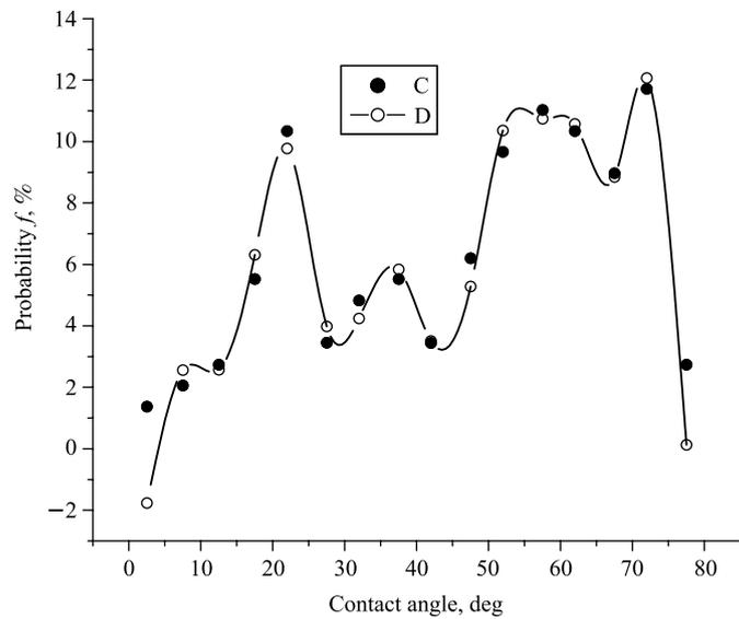
Fig. 3. OPEM approximation by 13th degree orthonormal polynomials (D) of non-treated water data (C)
