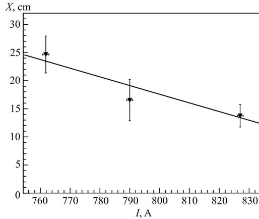
Fig. 10. The dependence of the  $X$ -position on the current in the last bending magnet of VP1 beamline. The line is the result of the fitting by the linear function
