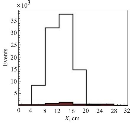
Fig. 6. The  $X$ -coordinate beam profile measured by scintillation hodoscope. The open and dashed histograms are the carbon and single charged particles, respectively
