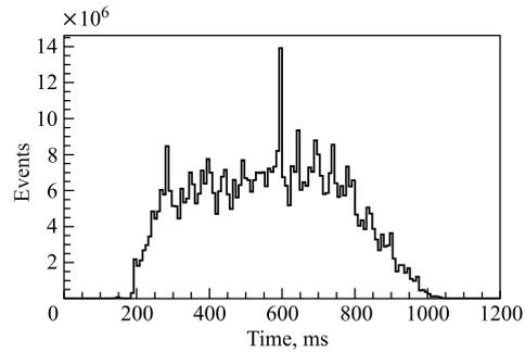
Fig. 9. The time distribution of the trigger signal appearance with respect to the beginning of the acceleration cycle
