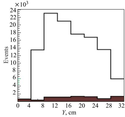
Fig. 7. The  $Y$ -coordinate beam profile measured by scintillation hodoscope. The histograms are the same as in Fig. 6
