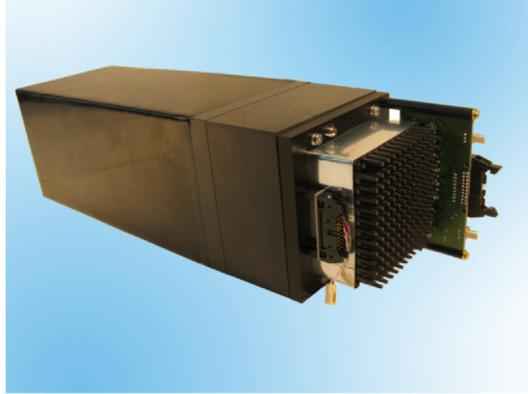
Fig. 2. View of the Shashlyk calorimeter module
