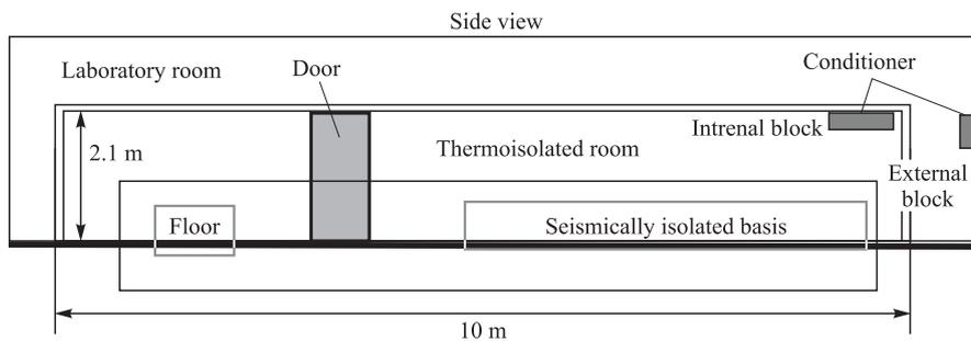
Fig. 1. The principal function scheme of the thermoisolated space (room) around seismically protected basis
