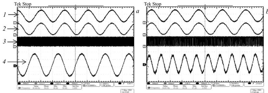
Fig. 3. The tube oscillations at first resonance frequency. Signals: 1 — Driver input; 2 — Excitation voltage control; 3 — Sensor high-frequency control signal; 4 — Sensor output signal proportional to the oscillation amplitude
