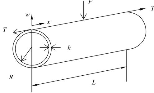
Fig. 2. Coordinate system of the tube and forces acting on it. Tube deviation  $w$  along the  $x$ -axis. Characteristics of the tube:  $R$  is the radius,  $L$  is the length,  $T$  is the tension, and  $F$  is the external oscillation excitation force
