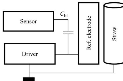
Fig. 1. Block diagram of the monitor
