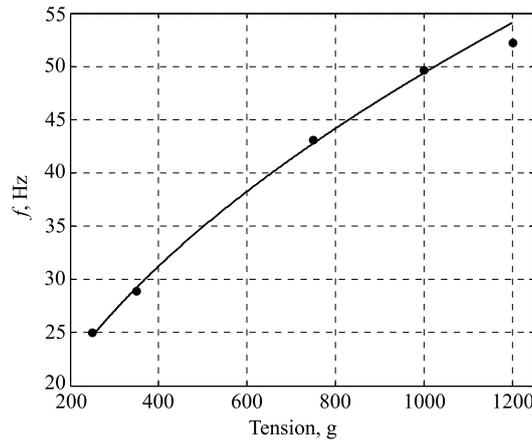
Fig. 5. Dependence of the resonance frequency on the tube tension
