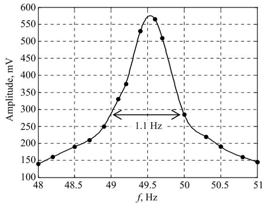
Fig. 4. Amplitude–frequency dependence of the readout signal
