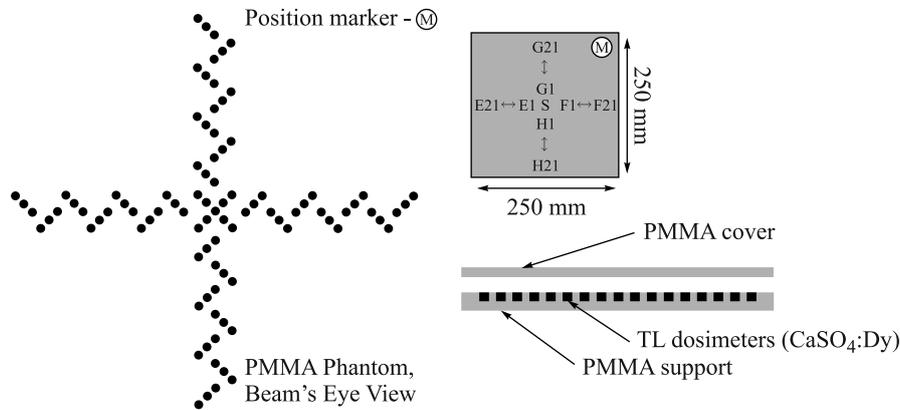
Fig. 1. Schematic drawing of the used phantom. Black dots represent holes for TLs
