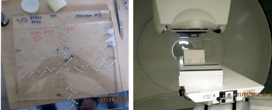
Fig. 2. Pictures of the PMMA phantom with TLDs (left) and gantry with the phantom (right)
