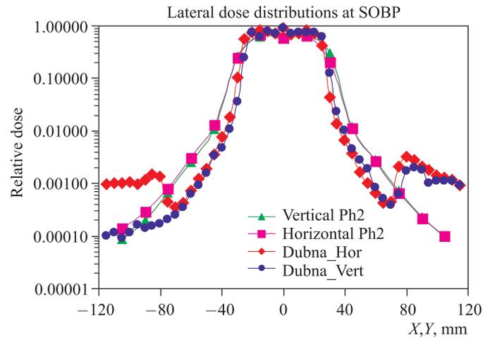
Fig. 7. Horizontal and vertical dose distributions measured in the Czech PTC, Prague, and in JINR, Dubna, at the centre of SOBP proton beams with  $\text{CaSO}_4:\text{Dy}$  TLDs
