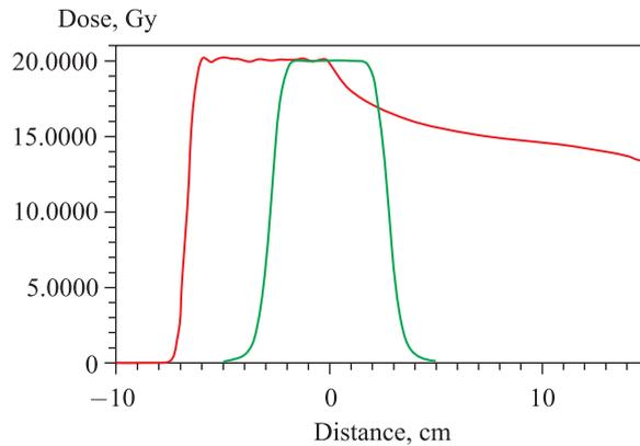
Fig. 3. Depth dose distribution and lateral profile of the PTC proton beam
