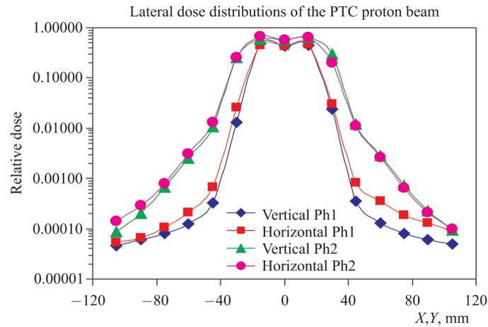
Fig. 4. Horizontal and vertical dose distributions measured in the PTC proton beam with  $\text{CaSO}_4:\text{Dy}$  TLDs
