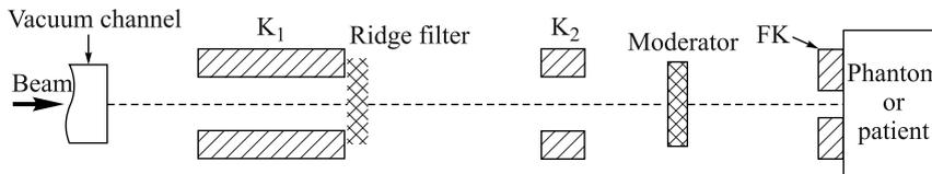
Fig. 5. Beam collimation system in the treatment room.  $K_1$  and  $K_2$  represent primary and intermediate collimators, FK represents the final shaping collimator
