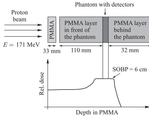
Fig. 6. Schematic drawing of the experiment, in which the phantom was positioned between two PMMA layers, and measuring the dose in the centre of the spread-out Bragg peak area
