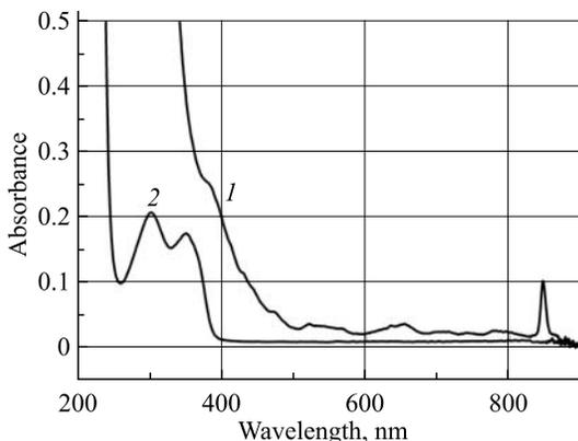
Fig. 7. Absorption spectra: 1 —  $\text{PuO}_2^{2+}$  (0.003 M) in solution 42% CsF +  $\text{H}_2\text{O}$ ; 2 — luminol (0.001 M) in solution 42% CsF +  $\text{H}_2\text{O}$ ; pH = 10.5
