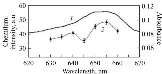
Fig. 12. Comparison of (1) the absorption spectrum of Pu(IV) and (2) the intensity of chemiluminescence at various wavelengths of radiation generated by the OBB-1012 dye laser (*two step–two color scheme*)
