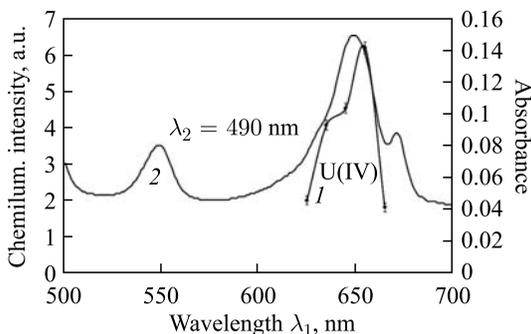
Fig. 10. 1 — spectrum of chemiluminescence excitation by the *two step-two color* scheme in luminol + U(IV) solution; 2 — absorption spectrum of U(IV) in aqueous HCl solution
