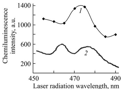
Fig. 9. 1 — spectrum of chemiluminescence excitation by the *two step-one color* scheme in luminol + Sm(III) solution; 2 — absorption spectrum of  $Sm^{3+}$
