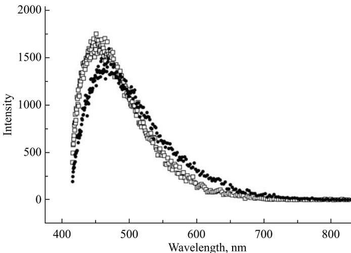
Fig. 6. Photoluminescence of  $\text{PuO}_2\text{F}_5^{3-}$  (0.001 M) + luminol  $10^{-4}$  M in CsF (42%) +  $\text{H}_2\text{O}$  (dots) and luminol  $10^{-4}$  M in CsF (42%) +  $\text{H}_2\text{O}$  (open squares). pH = 8.5. Excitation by pulsed (10 ns) nitrogen laser. 200 laser pulse were made per channel at spectrum measurement, laser beam diameter 5 mm, power in laser pulse 15 kW. Delay time 2  $\mu\text{s}$ . Gate time 50  $\mu\text{s}$
