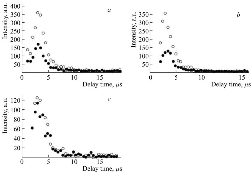
Fig. 4. Kinetics of luminol luminescence at the wavelength 459 nm in 42% solution of CsF in  $\text{H}_2\text{O}$ . pH: 8.19 (*a*), 9.86 (*b*), 11.85 (*c*). Open circles — without uranium, filled circles — 0.009 M of  $\text{UO}_2^{2+}$ . Luminol concentration  $10^{-4}$ . Gate time 1  $\mu\text{s}$
