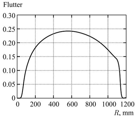
Fig. 4. Flutter along the radius
