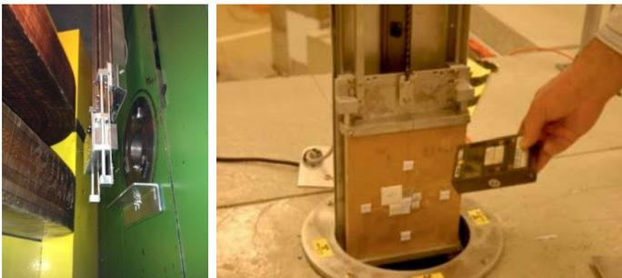
Fig. 6. Left: the lift on CUP position between magnet and collimator; right: the samples/foils on the paperboard on the upper lift position (outside the bunker)
