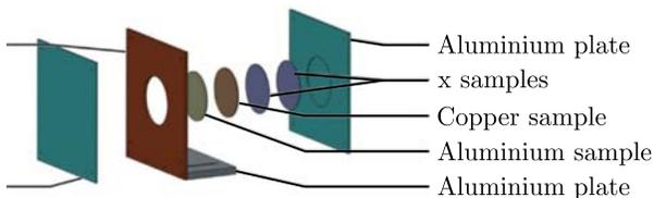
Fig. 5. Target stack arrangement for iTL irradiation
