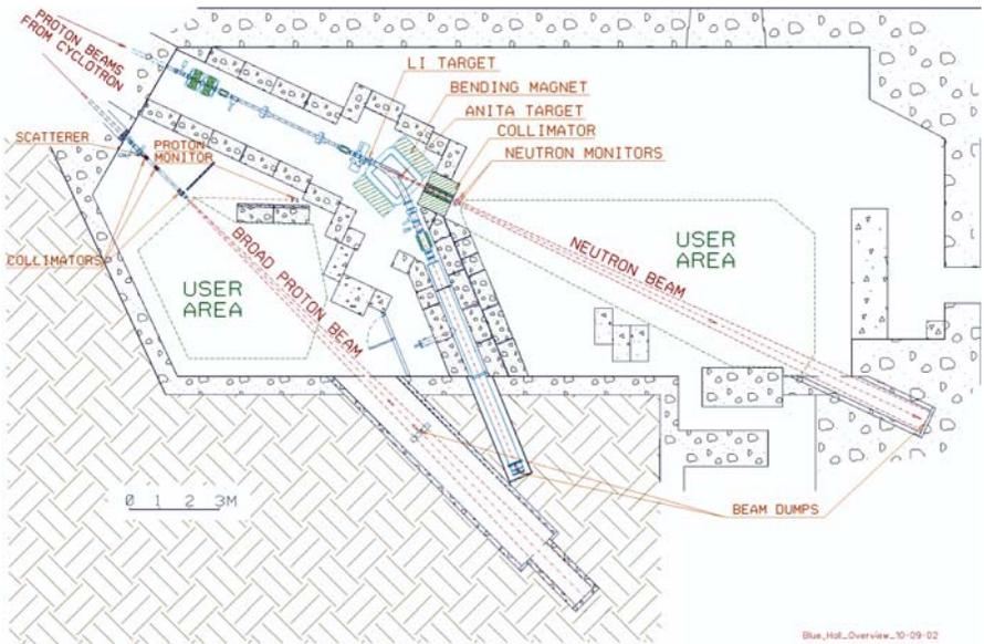
Fig. 4. The Blue Hall scheme. The CUP position is between the magnet and collimator
