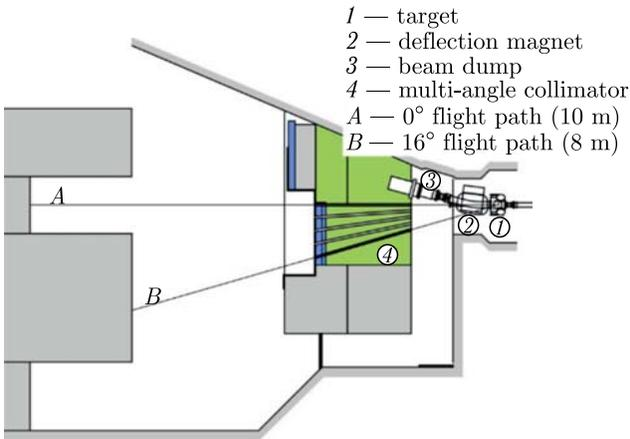
Fig. 3. Schematic view of the iThemba LABS neutron beam facility (drawn not to scale)
