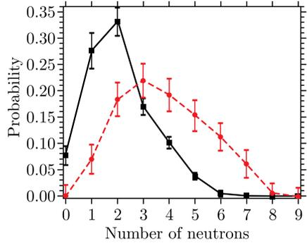
Fig. 6. Multiplicity distributions of the neutrons emitted in the spontaneous fission of  $^{246}\text{Fm}$ : detected in the experiment (squares) and reconstructed (circles). The lines connecting points have been added for clarity
