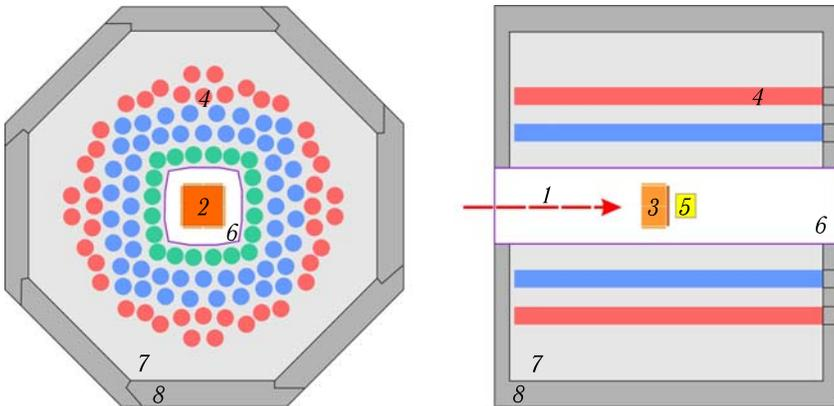
Fig. 2. The SFiNx scheme (front view — left; side view — right): 1 — recoil nuclei; 2 — focal-plane Si detector; 3 — tunnel Si-detector array; 4 —  $^3\text{He}$  counters; 5 — scintillator detector; 6 — vacuum chamber; 7 — moderator; 8 — shield
