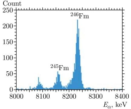
Fig. 4. Spectrum of  $\alpha$  particles obtained in the search for correlations with implanted recoil nuclei
