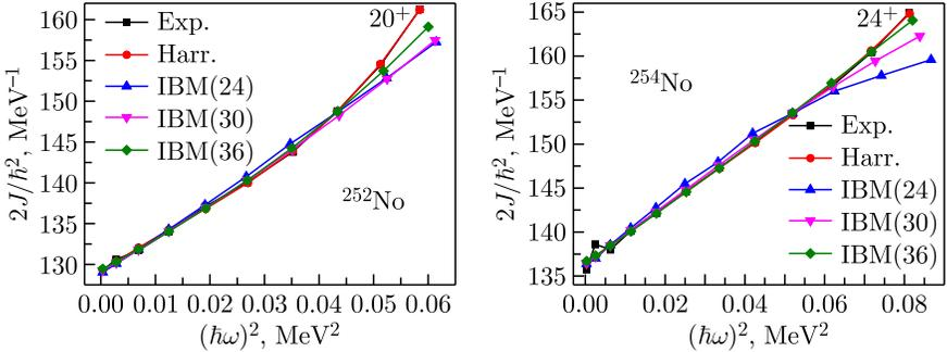
Fig. 8. Effective moments of inertia versus  $(\hbar\omega)^2$  for the yrast bands in No isotopes from experimental and theoretical energy values
