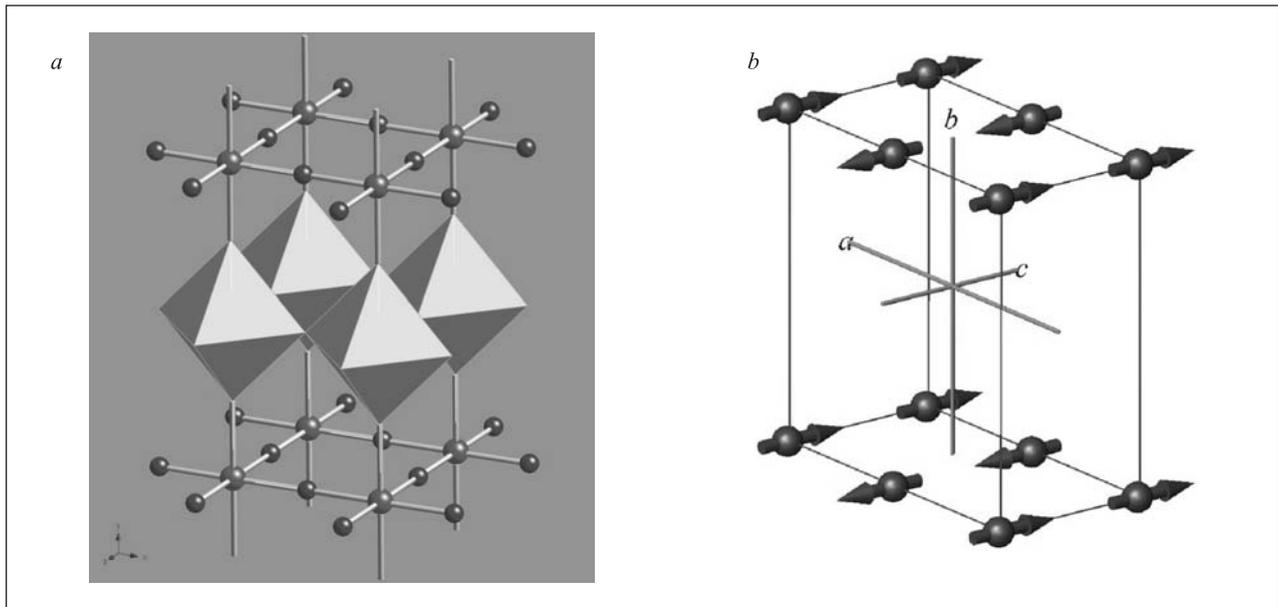
Fig. 1. The crystalline structure of  $\text{Sr}_2\text{GaMnO}_5\text{F}_1$  (a). The  $\text{MnO}_2$  planes and the  $\text{Ga}(\text{O},\text{F})_6$  octahedra are shown. The spin configuration in  $\text{Sr}_2\text{GaMn}(\text{O},\text{F})_6$  (b). Only the manganese are shown
