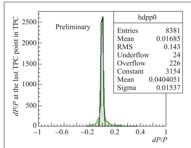
Fig. 6. The relative momentum resolution for charged particles
