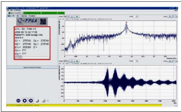
Fig. 10. A tune measurement using «Chirp» excitation (courtesy of the CERN AB/BI Group). The bottom trace shows the vertical beam response and the top trace is the spectrum of the signal with the vertical tune peak
