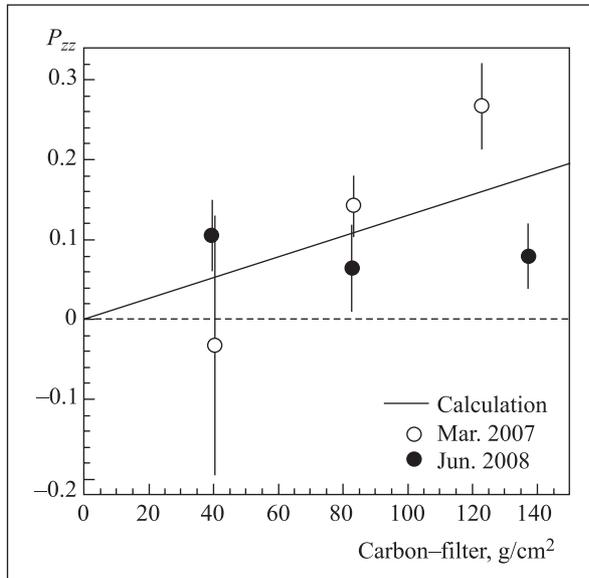
Fig. 3. Tensor polarization of deuterons vs thickness of the target. The dashed region shows the error values, the solid line is the theoretical prediction
