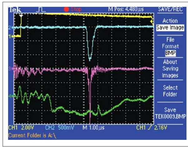
Fig. 1. The dependence of beam shifting (LUE-200, IREN) on the corrector field corresponds to the energy of electrons of 20 MeV. The current on the exit of the accelerator is 1.2 A (the upper curve). The signal of «Rogovsky belt» at the entrance to the target hall is 0.4 A (the middle curve). The amplitude line of RF field — the bottom curve
