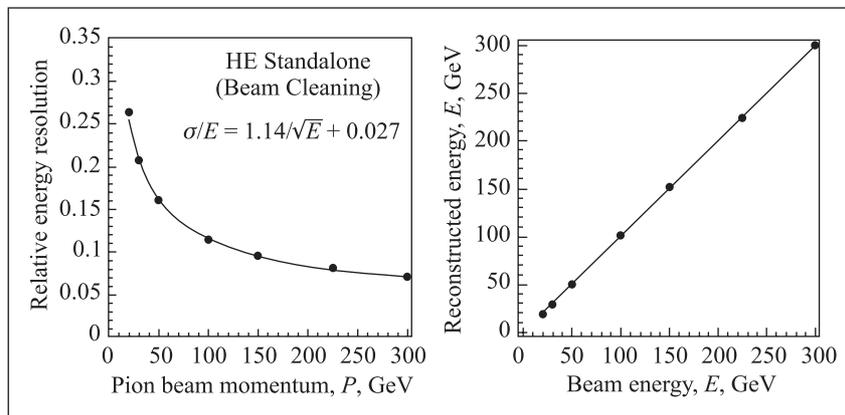
Fig. 4. The energy resolution (left) and ratio between the reconstructed and beam energy (right) for the combined end-cap calorimetry
