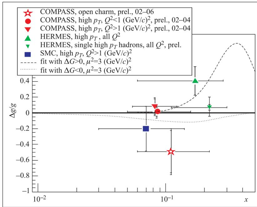
Fig. 2. Results of the  $\langle \Delta g/g \rangle_x$  measurements from the open charm and high  $p_T$  hadron pair production by COMPASS, SMC and HERMES as a function of Bjorken  $x$ . The curves display parameterizations from the NLO QCD analysis in the  $\overline{\text{MS}}$  scheme at  $Q^2 = 3$  (GeV/c)<sup>2</sup>: fits with  $\Delta G > 0$  (the broken line) and with  $\Delta G < 0$  (the dotted line)
