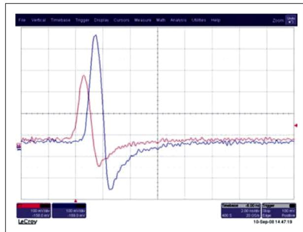
Fig. 9. Signals from the LHC Damper pick-up for the first shot of beam 2. The 10th of September 2008
