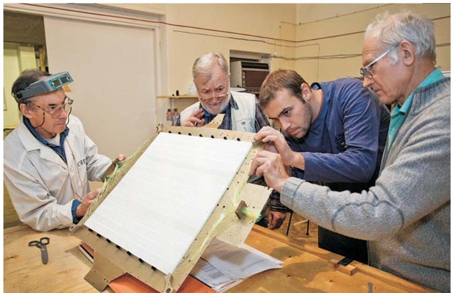
Dzhelepov Laboratory of Nuclear Problems. The assembly of the trigger module of the time-of-flight unit of the NUKLON detector
