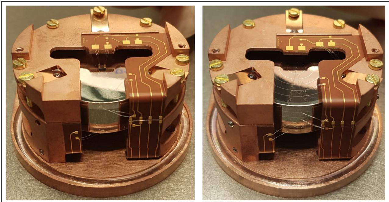
Fig. 2. Photos of a planar (left) and an FID (right) detector prototype made by EDELWEISS/Ricochet for Dark Matter search and precision study of CE $\nu$ NS
